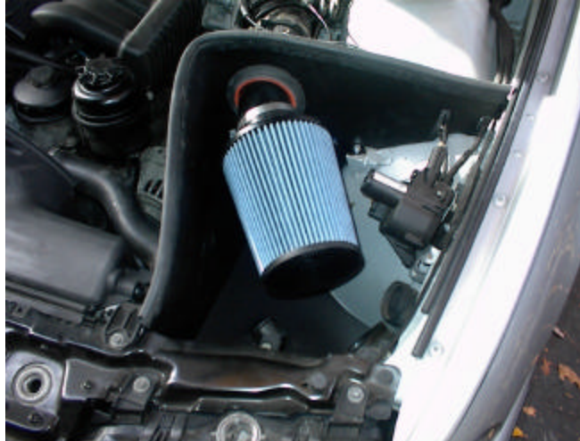
Shows Evolution Air Intake System installed on a 99 528
