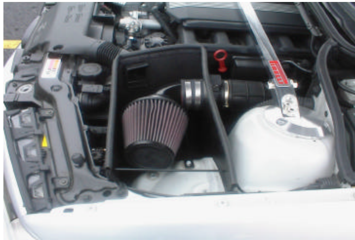
Shows Evolution Air Intake System installed on a 2000 323I
