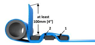
3. Check again for proper shoulder belt tilt lock adjuster positioning and for the 3bar slide to be as close as possible to the roll cage bar or end bracket.
