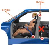
Never install shoulder belts directly to the floor behind the seat!
