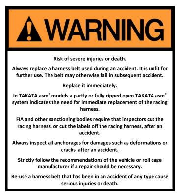
After an accident, in addition to replacing seatbelts which were in use, also ask your car dealer to carefully check all seatbelts attachment points for deformation or cracks. Always make sure the car manufacturer's guidelines are followed if a repair is necessary.
