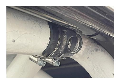
(2) Place **Long Mounting Tab** towards the front of the upper Bar either before or after the bend depending on the chassis it is going in. Miata's etc. before, Bmw's etc. after the bend. **See picture.**
