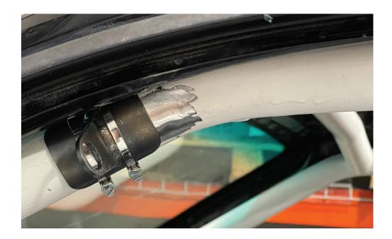
(3) Attach **Long Mounting Tab** with 2 Mounting band clamps with tab oriented so that it is pointing towards the side window. See picture.
