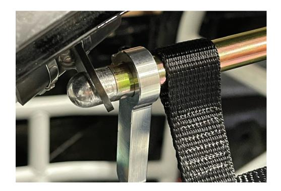
(4) Insert Spring Loaded Bar into net with the spring pin side oriented so it will be rearward.
