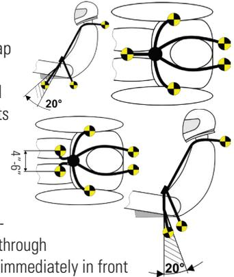
Note: FORMULA CARS where the driver is sitting on the sub-straps: Attach sub-straps rearwards in approximately the same location as the lap belts. This type of setup is typically used with a "Formula Style" or "Hybrid Style" looped sub-strap.
