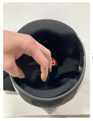
2) Remove the left cheek pad. The chin pad will be removed and replaced with the new one.
