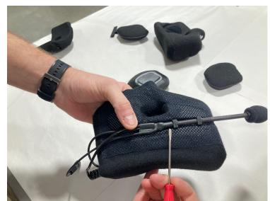
5.1) Place the mic into the cheekpad tray while keeping in mind the "TALK" orientation on the microphone. The edge of the last stem block should be in line with the edge of the chin strap outlet.
