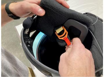
7) Place the extra speaker wire and cup outside of the shell then pull the chin strap through the cheek pad and secure. The chin pad can be installed back into the helmet anytime between steps 7 and 9.
