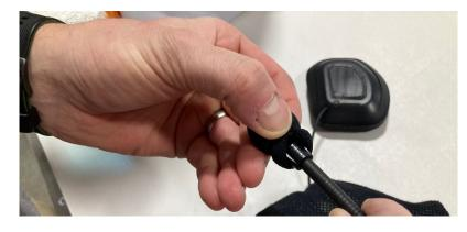
5) Locate the word "TALK" on the Mic Boom. This is the side that will be facing the user. This orientation is important to get correct.
