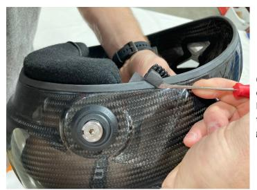
6) Find the connector tether and work the clip onto the rubber seal around the bottom. It is recommended to take your time and use a small screwdriver to help guide the part over the seal.
