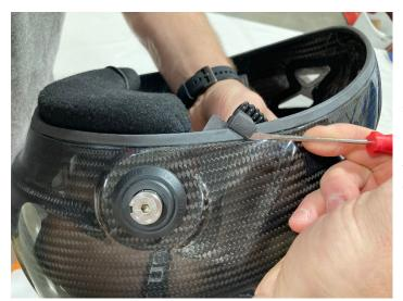
4) Find the connector tether and work the clip onto the rubber seal around the bottom. It is recommended to take your time and carefully use a small screwdriver to help guide the part over the seal.
