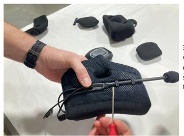
3.1) Place the mic into the cheek pad tray while keeping in mind the "TALK" orientation on the microphone. The edge of the last stem block should be in line with the edge of the chin strap outlet.
