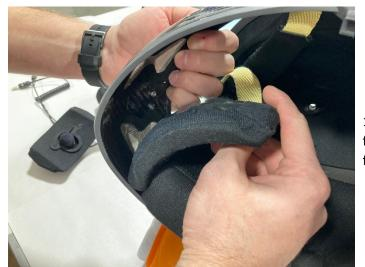
10) Install a cheek pad, then the chin pad followed by the remaining cheek pad. Don't forget the chin straps!
