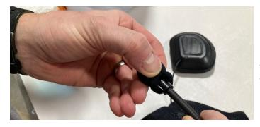
3) Locate the word "TALK" on the Mic Boom.This is the side that will be facing the user.This orientation is important to get correct.
