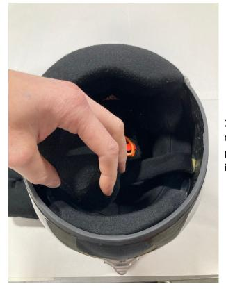
2) Remove the cheek pad of the side you wish to have the microphone placed on. The chin pad can also be removed to help with the installation if you wish.
