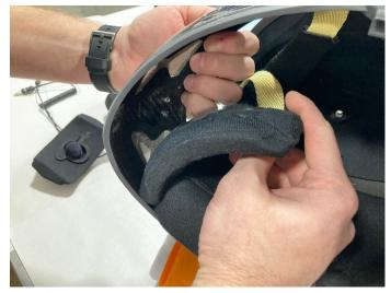
3) Remove the chin pad and loosely place the equipment into the helmet
