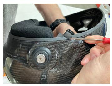
4) Find the connector tether and work the clip onto the rubber seal around the bottom. It is recommended to take your time and carefully use a small screwdriver to help guide the part over the seal.
