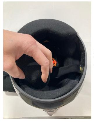
2) Remove the right cheek pad. The chin pad will be removed and replaced with the new one.
