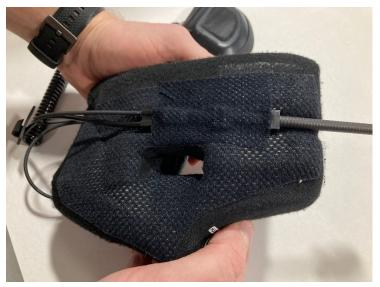
5.2) Place the included strip of nomex tape over top of the microphone boom to help hold it and place all of the equipment into the helmet for step 6.
