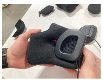
4.1) This denotes that it is the Right earcup and should be installed into the right cheekpad with UP towards the top of the helmet.
