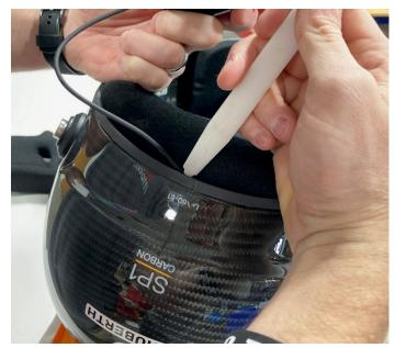
8) Secure the speaker wire in around the back of the helmet by tucking it in with a blunt tool as shown.
