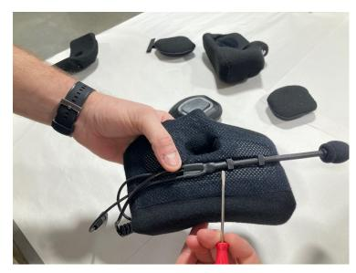
5.1) Place the mic into the cheekpad tray while keeping in mind the "TALK" orientation on the microphone. The edge of the last stem block should be in line with the edge of the chin strap outlet.
