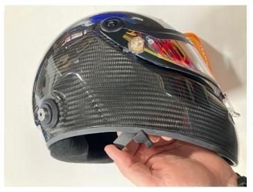
7) In the same manner as in step 6 and 6.1, carefully install the earbud clip and move into place wherever is most comfortable for the driver.
