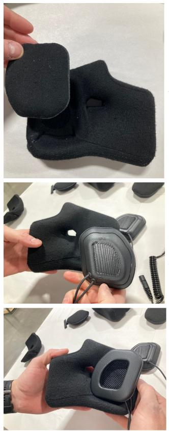
3) Remove the ear pads from the chin pads. They are secured with small pieces of velcro.
