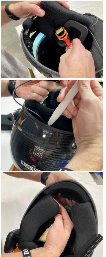
8) Place the extra speaker cup and earbud wire outside of the shell then pull the chin strap through the cheek pad and secure. The chin pad can be installed back into the helmet anytime between steps 7 and 9.
