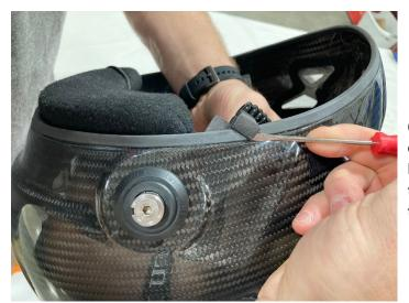
6) Find the connector tether and work the clip onto the rubber seal around the bottom. It is recommended to take your time and carefully use a small screwdriver to help guide the part over the seal.
