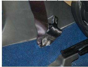
Reinstall the carpet allowing the Schroth piece and factory belt to come out of the pre-cut hole in the carpet. Reinstall all factory molding and pieces in the reverse order of disassembly.
