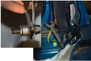
Mount the SCHROTH bracket as shown in the picture above left. Be sure to use the STi hardware, bolt, washer, and spacer as pictured above.
