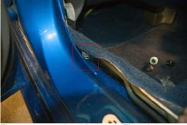
☐ The carpet must be pulled back. There is a small clip that holds the carpet in place, slide it forward.
