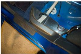
☐ Remove small plastic retaining tab.
