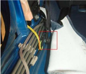
Locate and remove (using a 14mm socket) the outermost lap belt anchor bolt.
