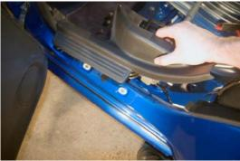
☐ Plastic Piece is held in with tension clips Pull up in a vertical plane to remove.
